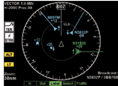
Received by a universal access transceiver, this traffic information service displays a 3-D picture of traffic relative to position.
