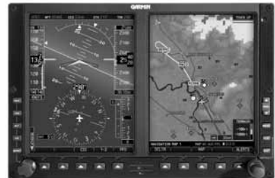
The Garmin G600 all-glass flight display system replaces the standard six-pack. All of the functions of a PFD and MFD are placed directly in front of the pilot.
